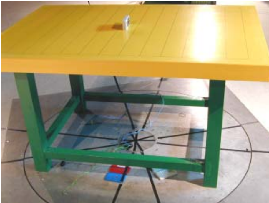
Photo 2: Radiated Emission Test Set-up
