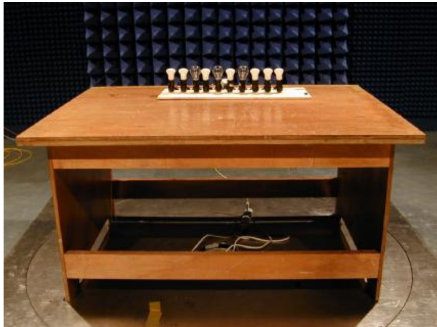
Photo 2: Radiated Emission Test Set-up (WL-902)
