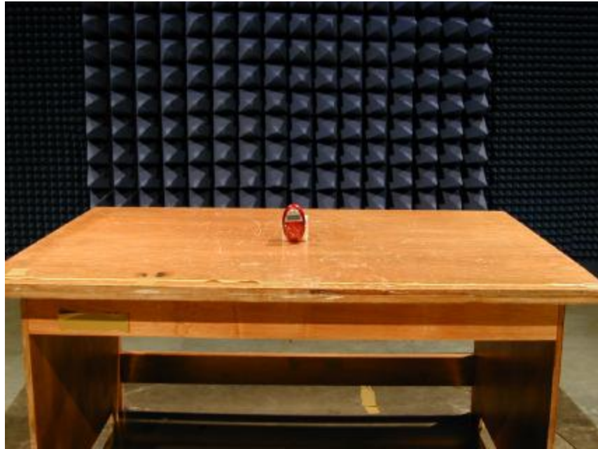
Photo 2: Radiated Emission Test Set-up (WL-902)
