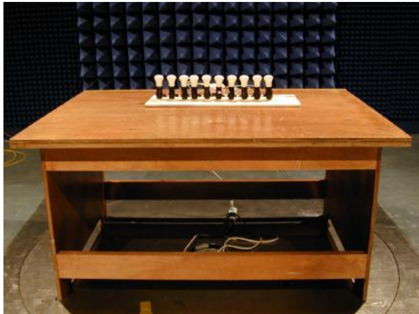
Photo 4: Radiated Emission Test Set-up (WL-905)
