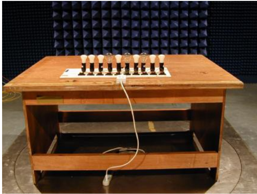
Photo 4: Radiated Emission Test Set-up (WL-905)
