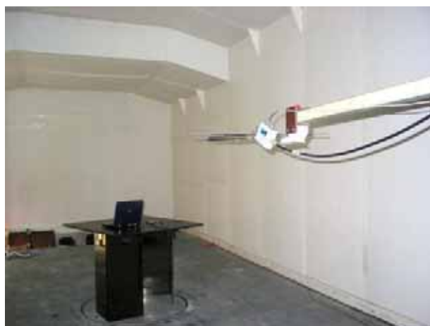
Radiated Emissions Measurement in Open Area Test Site Frequency range: 200 MHz – 1 GHz Configuration: WDP318 connected to laptop PC and earphone
