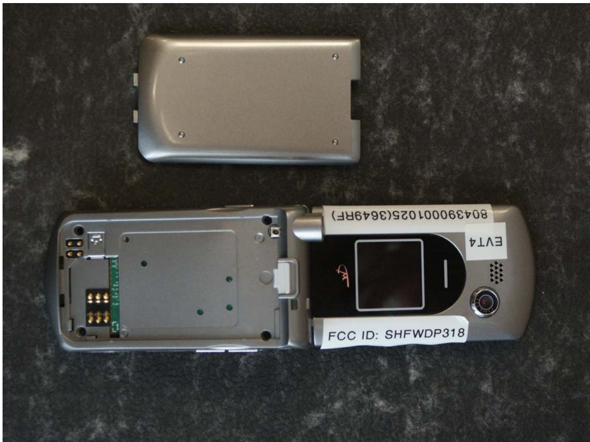
Photo 6. Back view with battery removed
