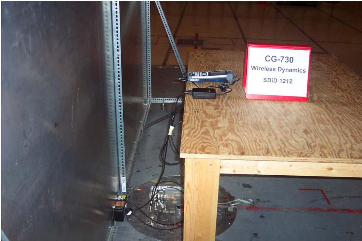
Figure 4 Conducted Emissions Test Photograph 2 (150 kHz – 30 MHz)
