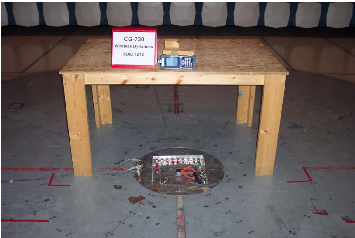
Figure 2 Radiated Emissions Test Photograph (9 kHz – 30 MHz)
