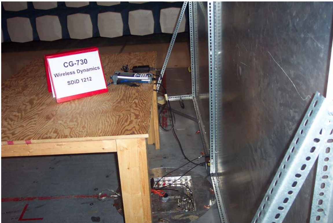
Figure 3 Conducted Emissions Test Photograph 1 (150 kHz – 30 MHz)
