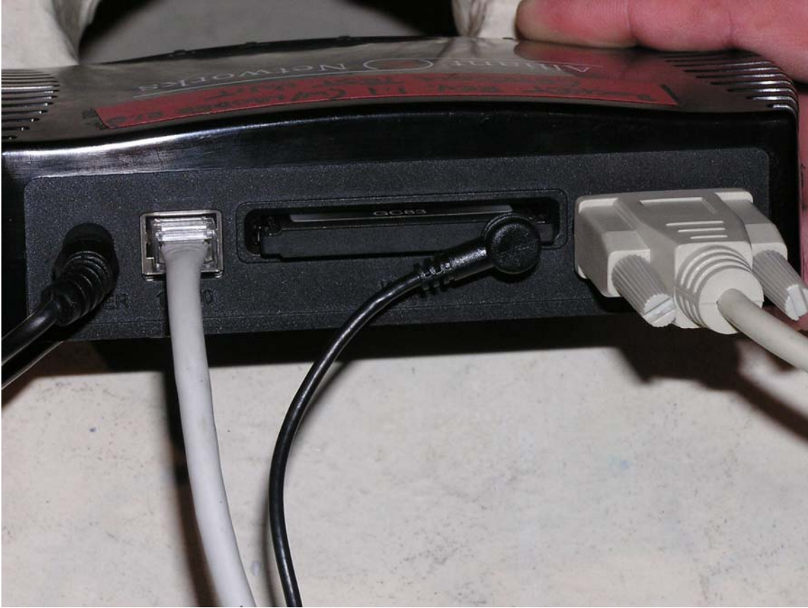
EUT with GSM card in PCMCIA slot
