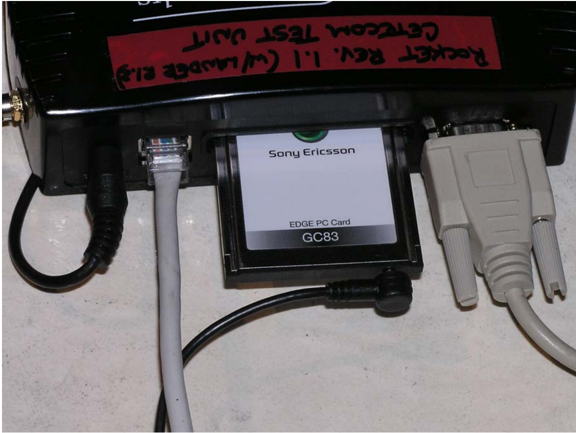
EUT with GSM card in PCMCIA slot
