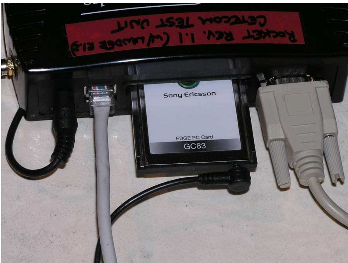
EUT with GSM card in PCMCIA slot
