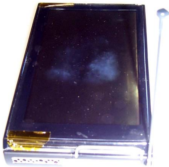
Fig. 1: Intended operation position of WLAN swivel antenna with whip oriented vertically.
