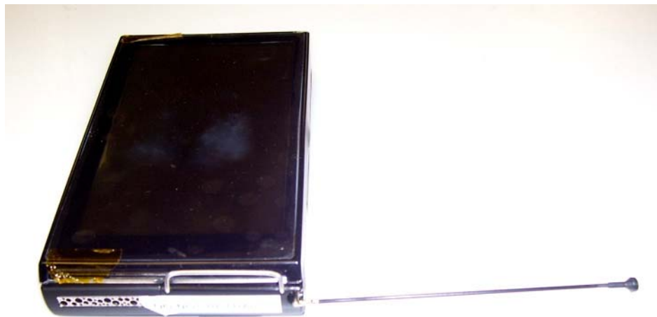
Fig. 2: Extreme position of swivel antenna
