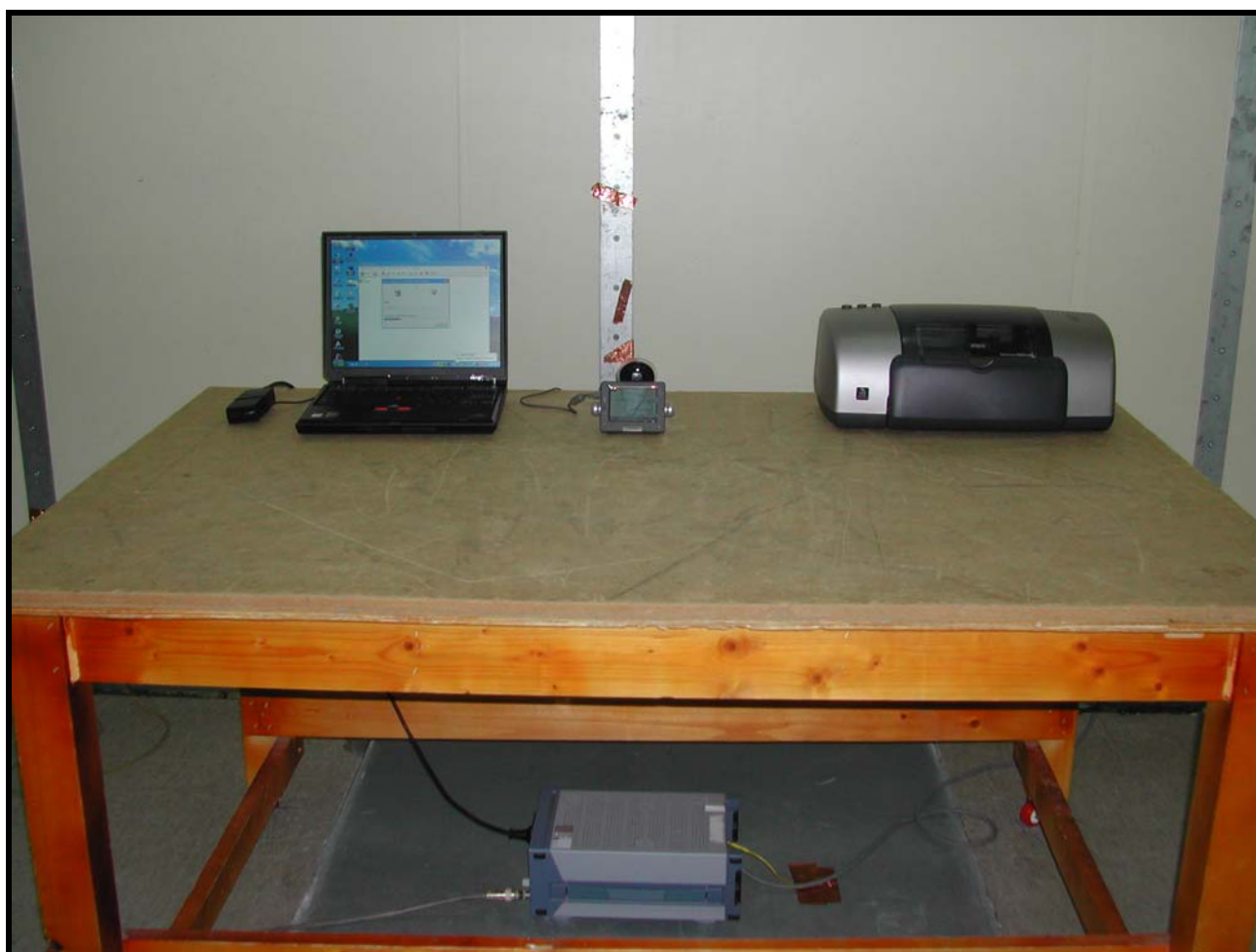
Photograph 1: Setup for Conducted Emissions
