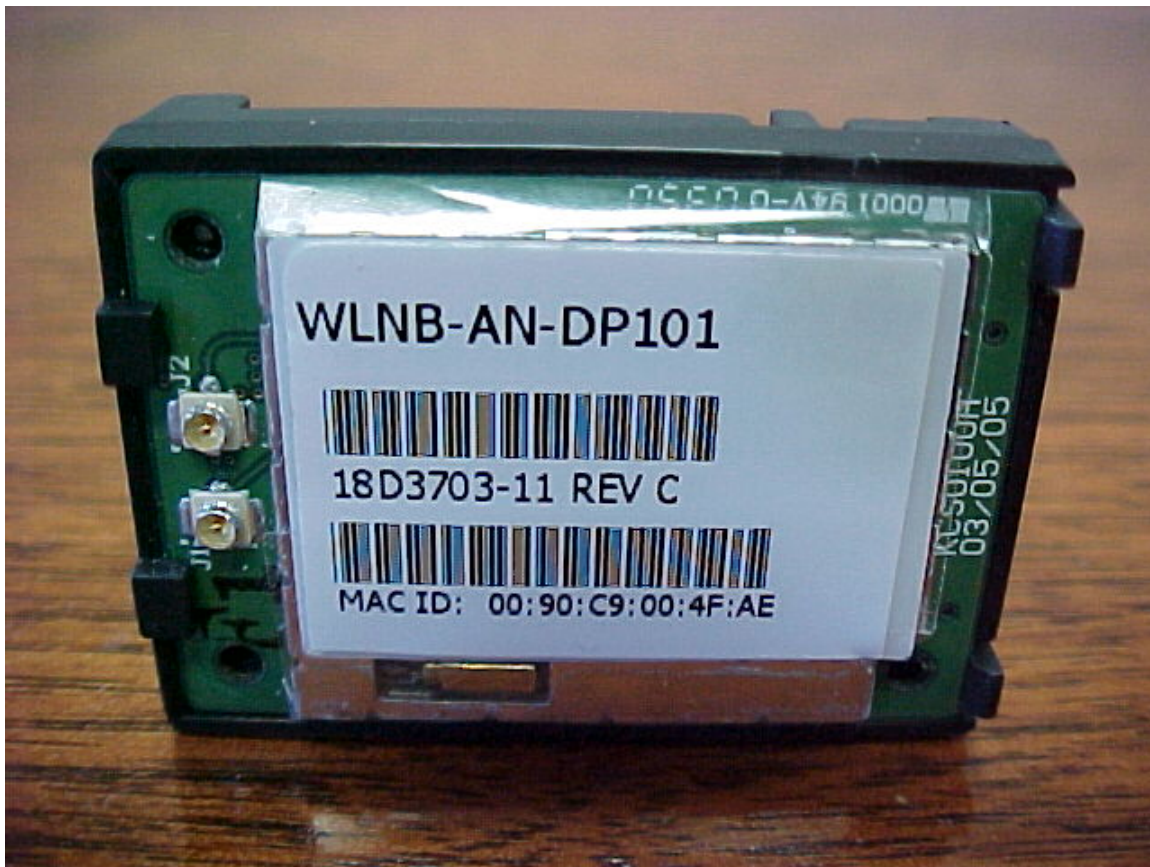
Photo Four – Internal RF Module, prepackaged by DEPAC Airborne Wireless
