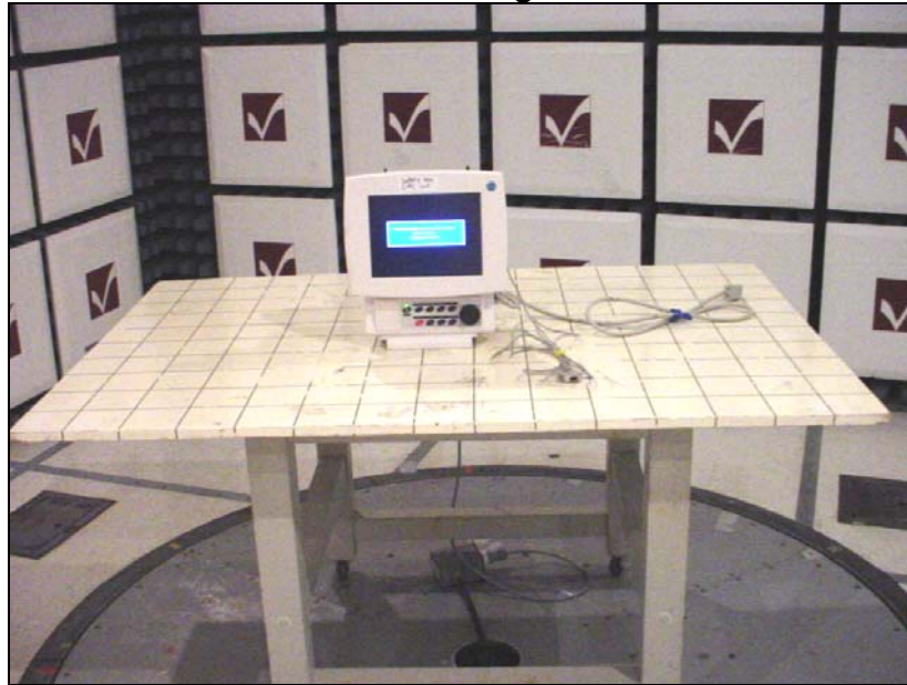
View of the 'Remote' EUT during radiated emissions test
