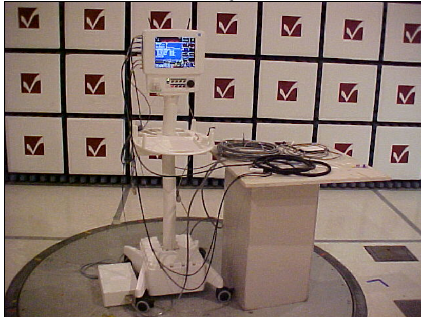
View of the 'Main' EUT during radiated emissions test
