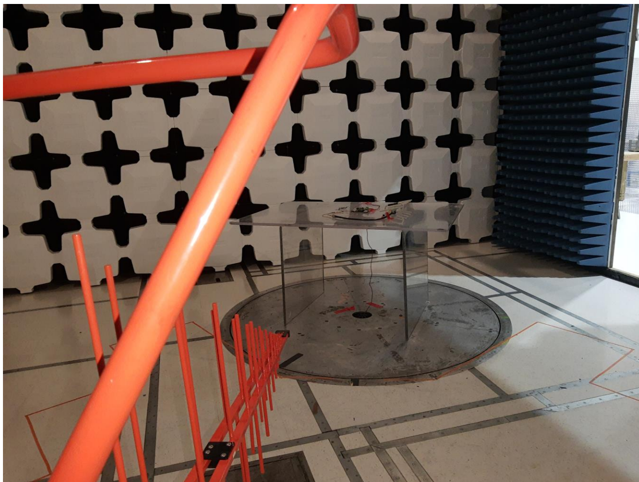
Figure 3: Radiated Emissions Test Setup - 30-1000MHz - 12dBi configuration
