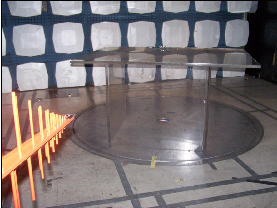
Photograph 6. Radiated Spurious Emissions, Test Setup, 1 dBi Antenna
