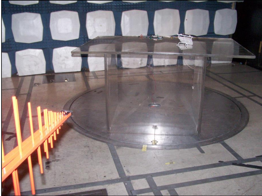
Photograph 8. Radiated Spurious Emissions, Test Setup, 12 dBi Antenna
