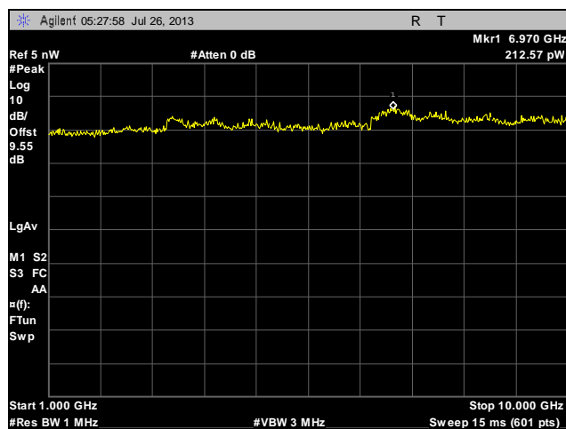
Plot 274. Receiver Spurious Emission, 250 kbps, 250 kHz, High Channel, 1 GHz – 10 GHz, 1 dBi Antenna
