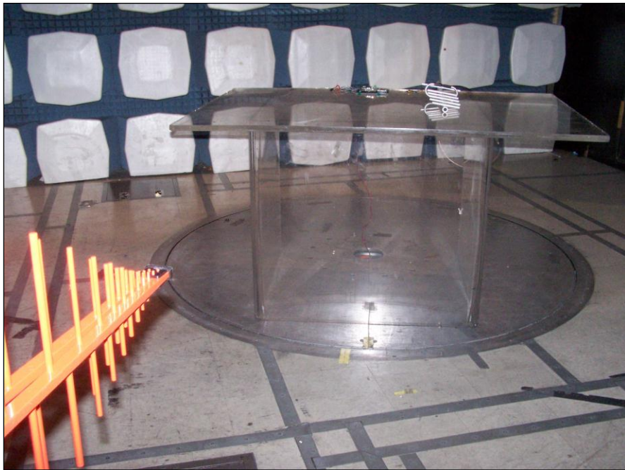
Photograph 2. Radiated Emission, Test Setup, 12 dBi Antenna
