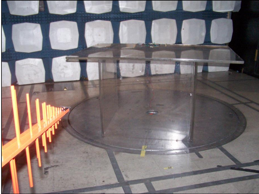
Photograph 3. Radiated Spurious Emissions, Test Setup, 1 dBi Antenna
