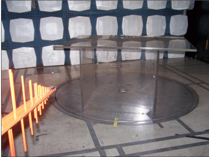
Photograph 1. Radiated Emission, Test Setup, 1 dBi Antenna
