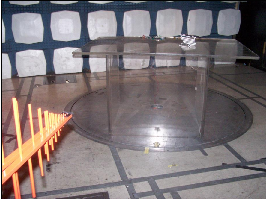
Photograph 5. Radiated Spurious Emissions, Test Setup, 12 dBi Antenna
