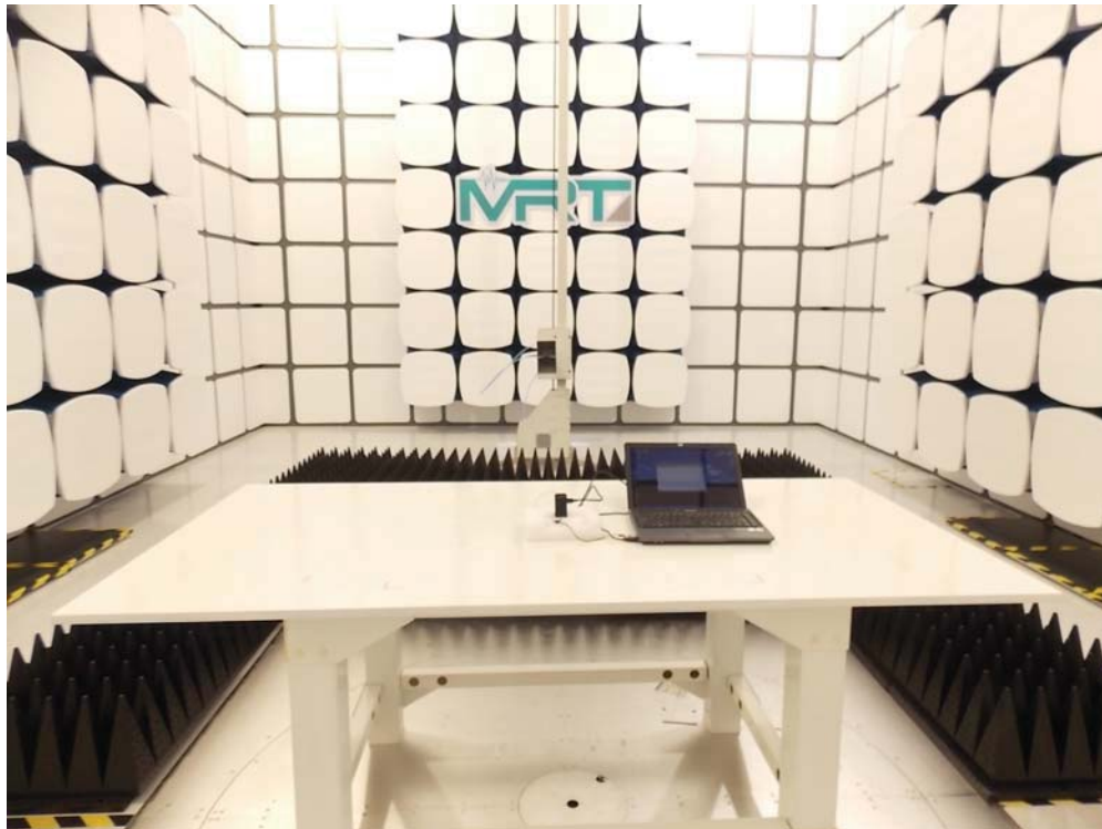
Description: Radiated Emission Test Setup for 1~18GHz
