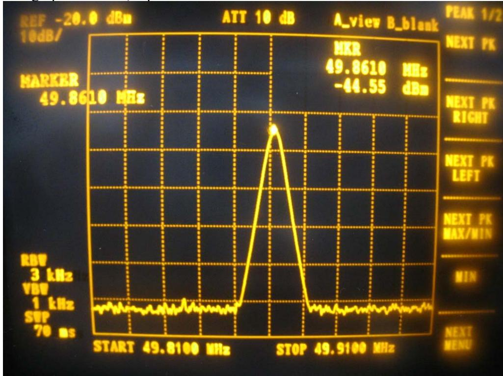
**The results: The unit does meet the FCC Part 15 C Section 15.235 requirements.**
