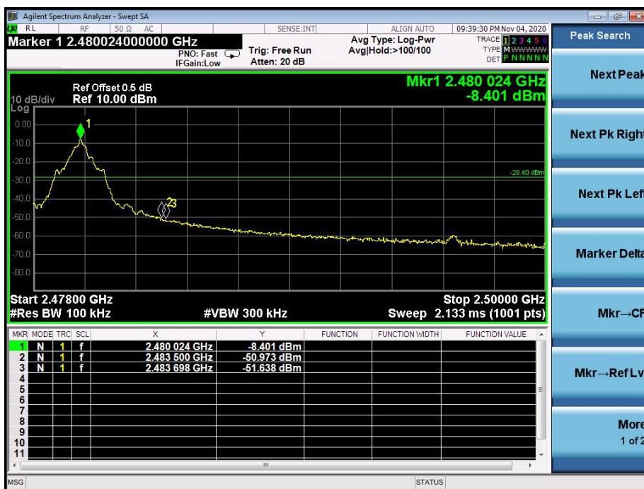
GFSK: Band Edge, Right Side
