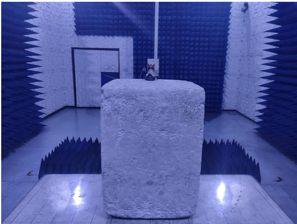
RADIATED EMISSION TEST SETUP ABOVE 1GHz
