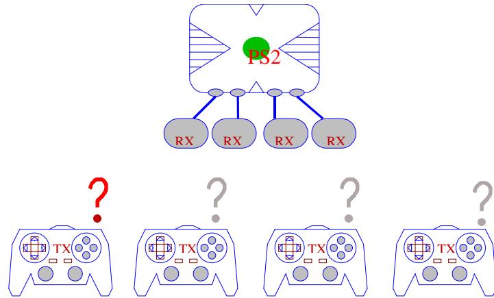
In this situation, please turn off all the controllers power, Then turn on one of controller power and press AC key. So new channel will confirm and Connect LED in the receiver and controller will light.
