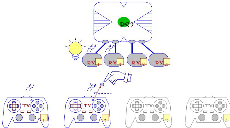
c). In the situation that receiver's ID is different from controller's
