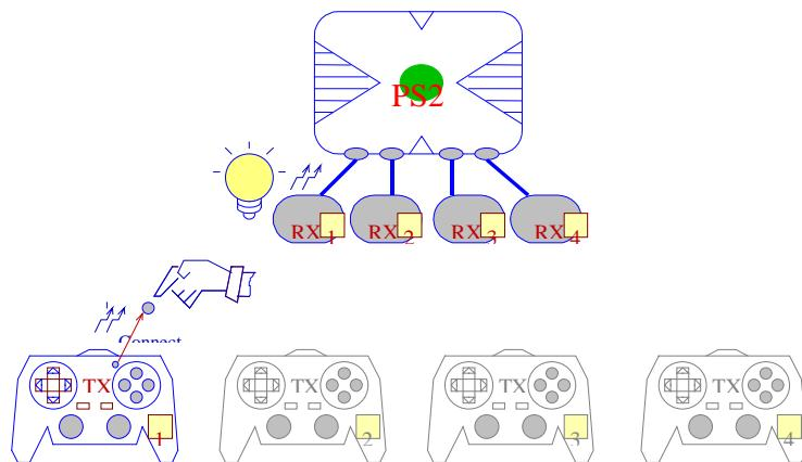
Turn on the next controller power and press AC key, so this channel will confirm and CONNECT LED light. In this way you can reset the rest channels in turn.
