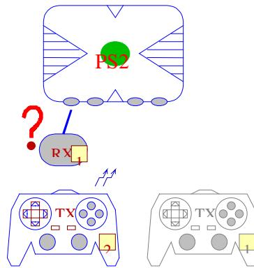
Press AC key of receiver, then press the AC key of your wished controller. After that, ID resetting has completed. At the same time, channel will confirm and CONNECT LED lights. So you can play normally.
