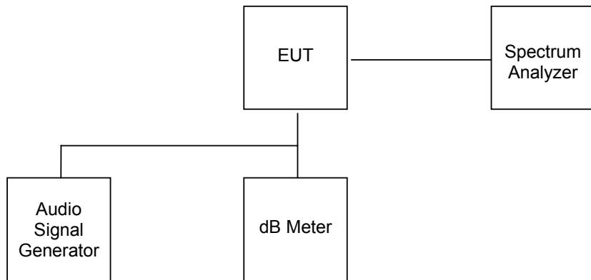
2. Other than single side band or independent sideband transmitters when modulated by a 2500Hz one at an input level 16dB greater than that necessary to produce 50 percent modulation. The input level shall be established at the frequency of maximum response of the audio modulating circuit.
