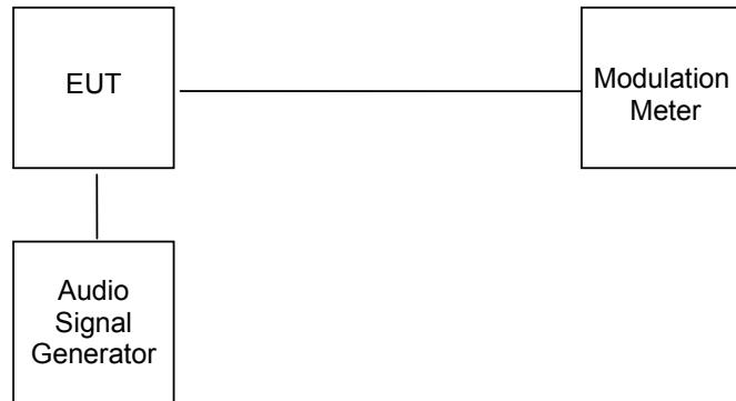
2. Set the frequency of the audio signal generator to 500Hz and adjust the level from 67dB SPL to 127dB SPL. Record the output modulation index.
