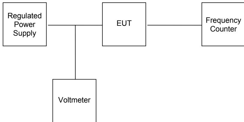
2. For battery powered equipment, reduce primary supply voltage to the battery operating end point voltage which is specified by the manufacturer.
