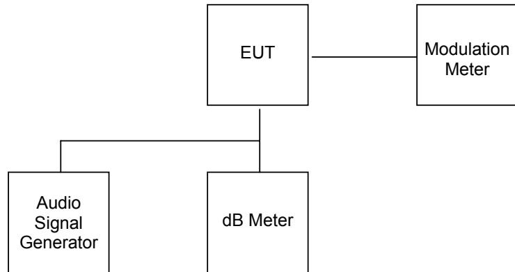
2. Set the audio signal generator frequency to the sound pressure level 97.0dB SPL at the microphone of the EUT.
