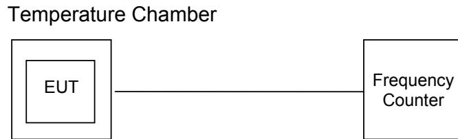
2. Set the Temperature Chamber to -30°C and stabilize the EUT temperature for one hour. Turn the transmitter ON for two minutes.
