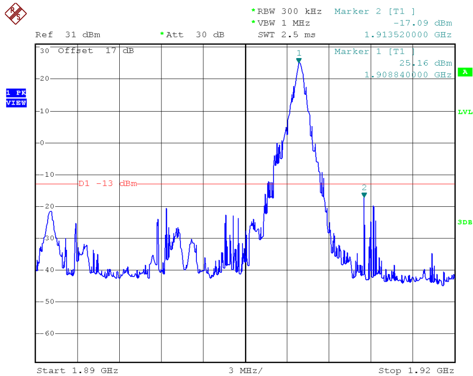
Higher Band Edge Plot for 16QAM-RB Size 1, RB Offset 99
