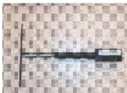
Figure 1 – Satimo COMOSAR Validation Dipole
