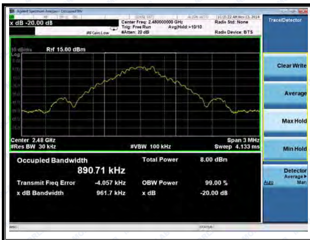
(Plot C: Channel = 2480 @ GFSK)
