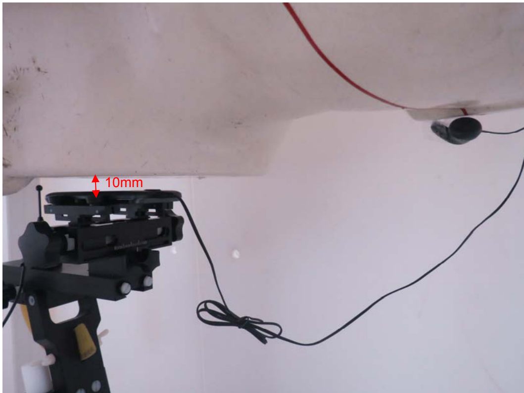
Picture 19: Back Side with earphone 1, the distance from handset to the bottom of the Phantom is 10mm
