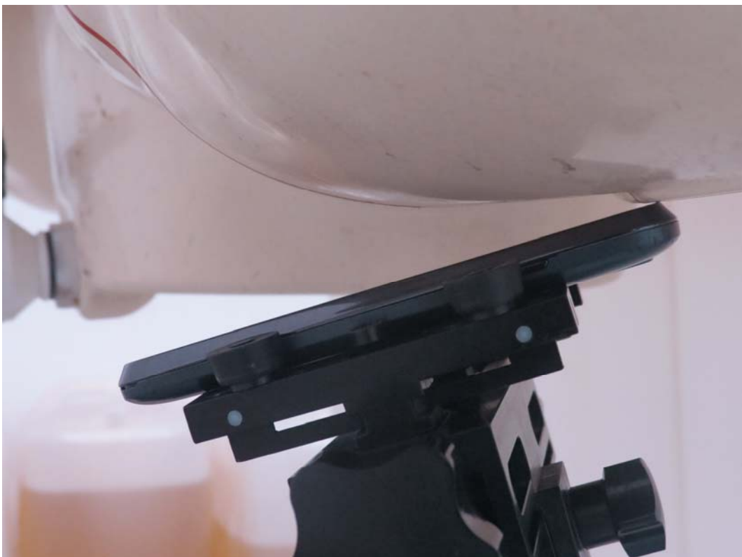
Picture 10: Left Hand Tilt 15 Degree Position
