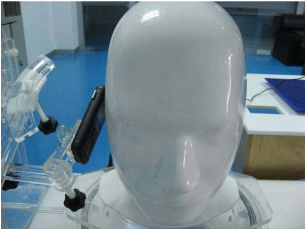
Fig.4 EUT Left Head Tilt15 Position
