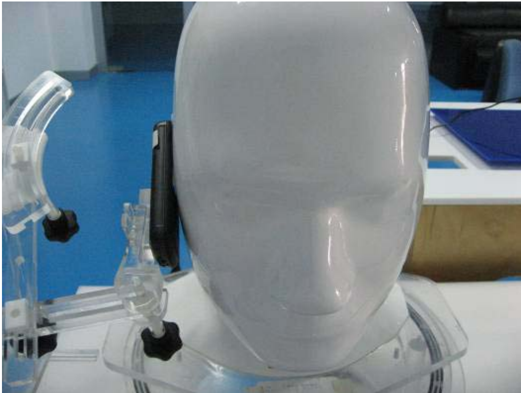
Fig.3 EUT Left Head Touch Cheek Position
