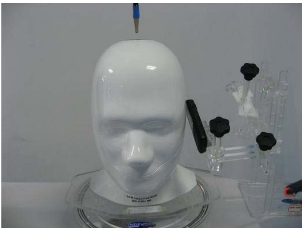
Fig.6 EUT Right Head Tilt15 Position
