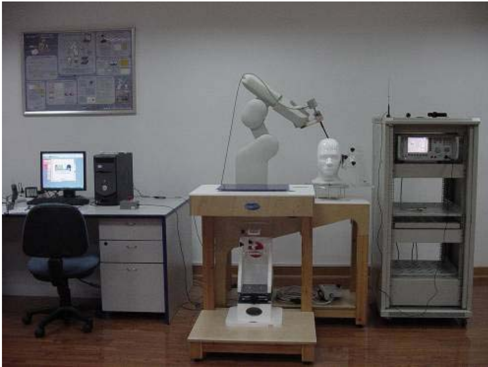
Fig.1 SARA2 System Test Layout
