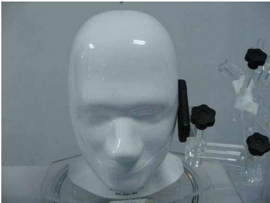
Fig.5 EUT Right Head Touch Cheek Position
