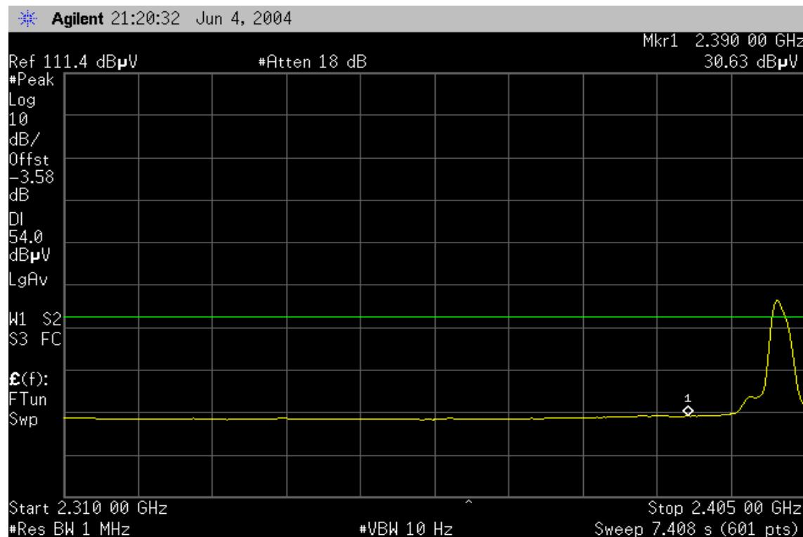
**Band Edges Test Data (CH-High)****Detector mode: Peak****Polarity: Vertical**
