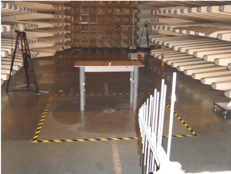
Set-up for Radiation Emission (Transceiver)
