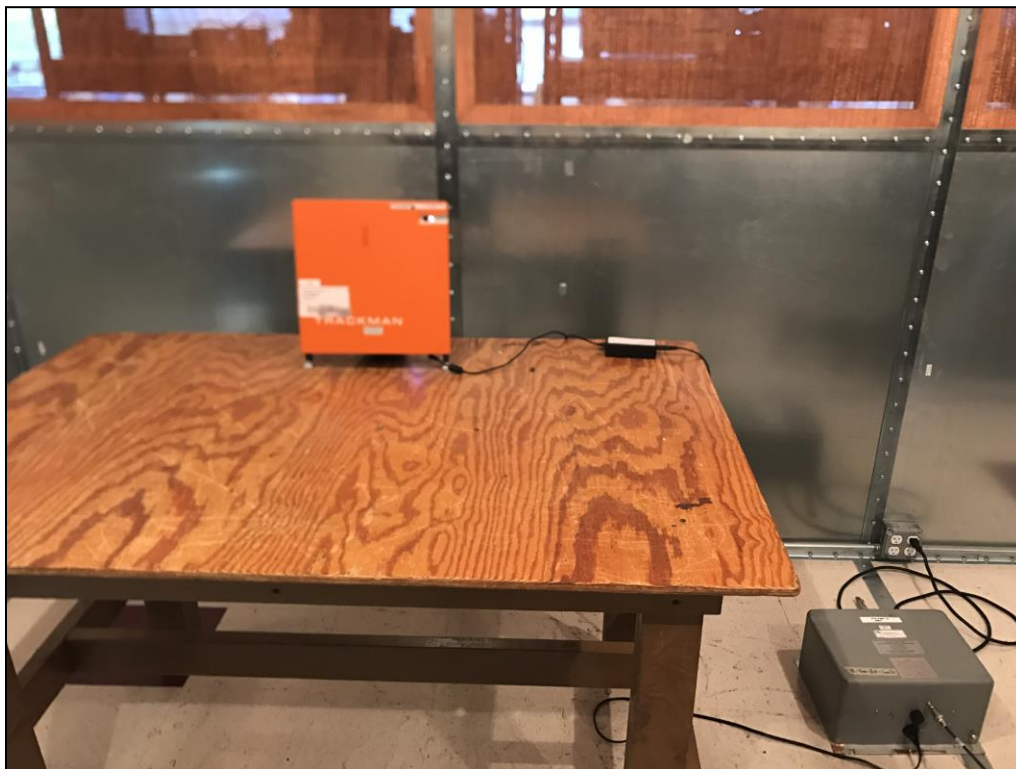
Photograph 1. Conducted Emissions, 15.207(a), Test Setup
