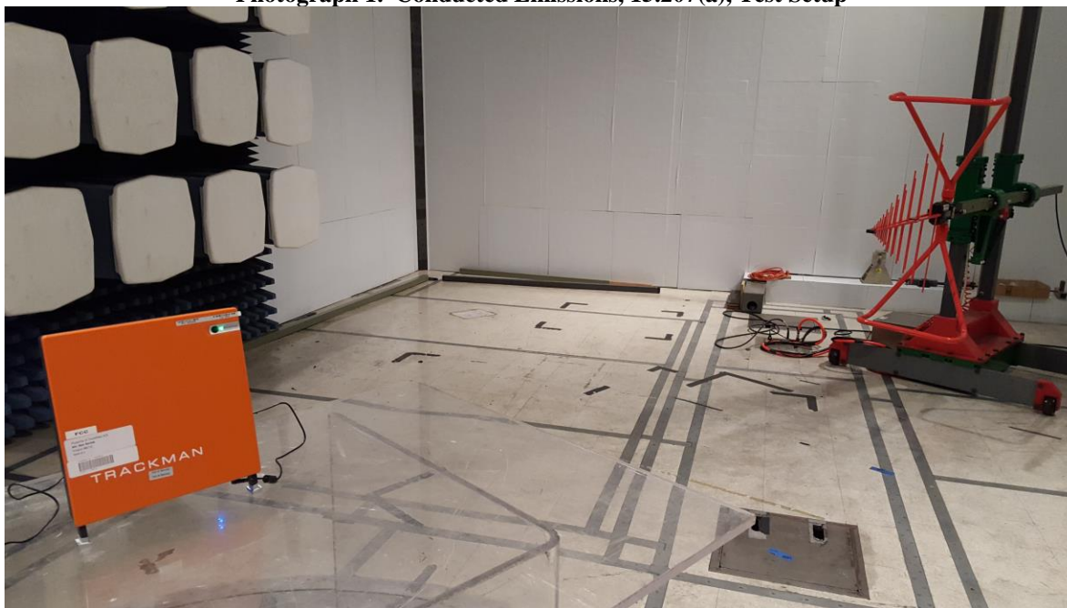
Photograph 2. Radiated Spurious Emissions, Test Setup, Below 1GHz
