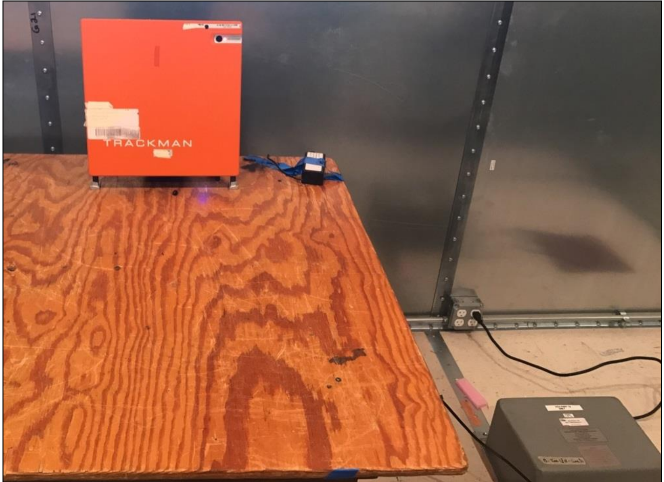
Photograph 1. Conducted Emissions, 15.207(a), Test Setup
