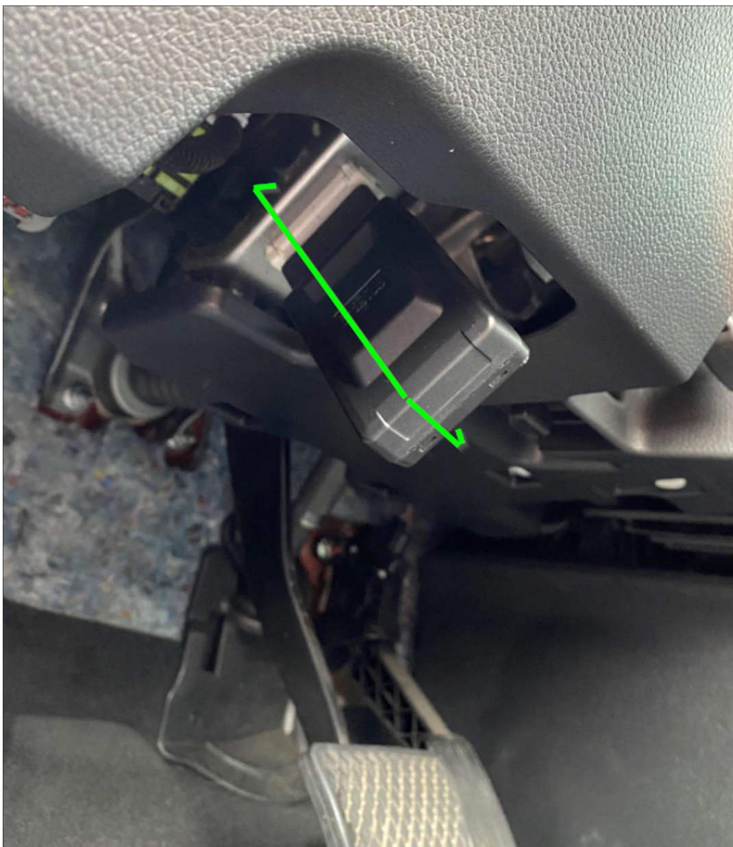
Figure 4 - Suggested place (in green) to hold back with a tie wrap
