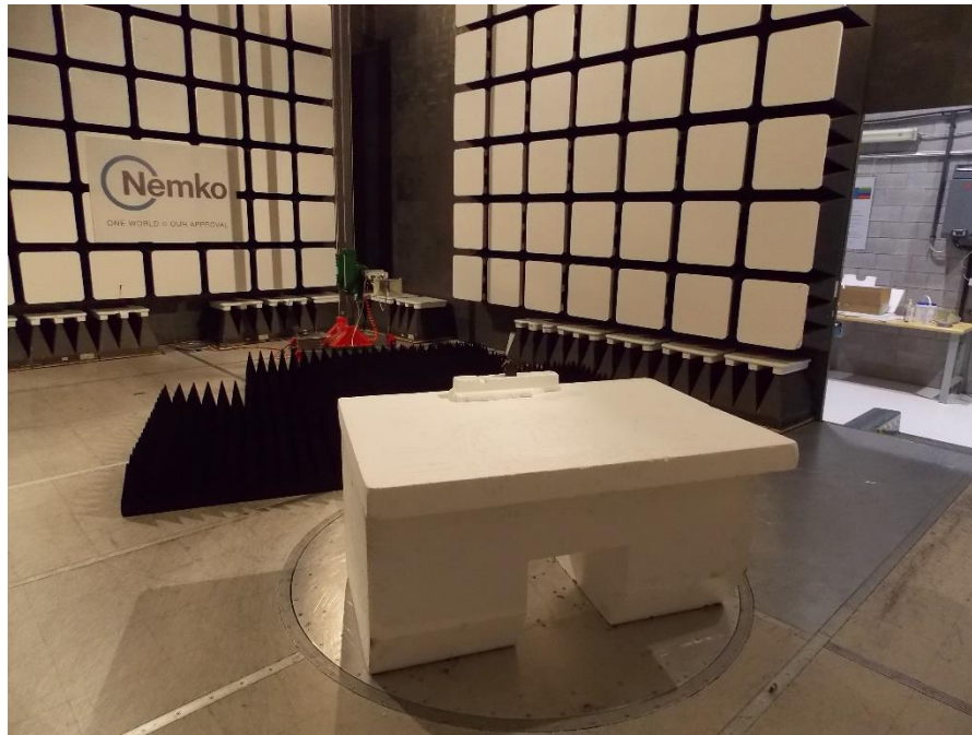
Figure 8.1-7: Radiated emissions setup photo – above 1 GHz
