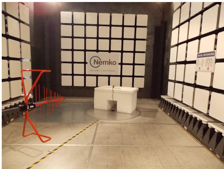
Figure 8.1-6: Radiated emissions setup photo – below 1 GHz
