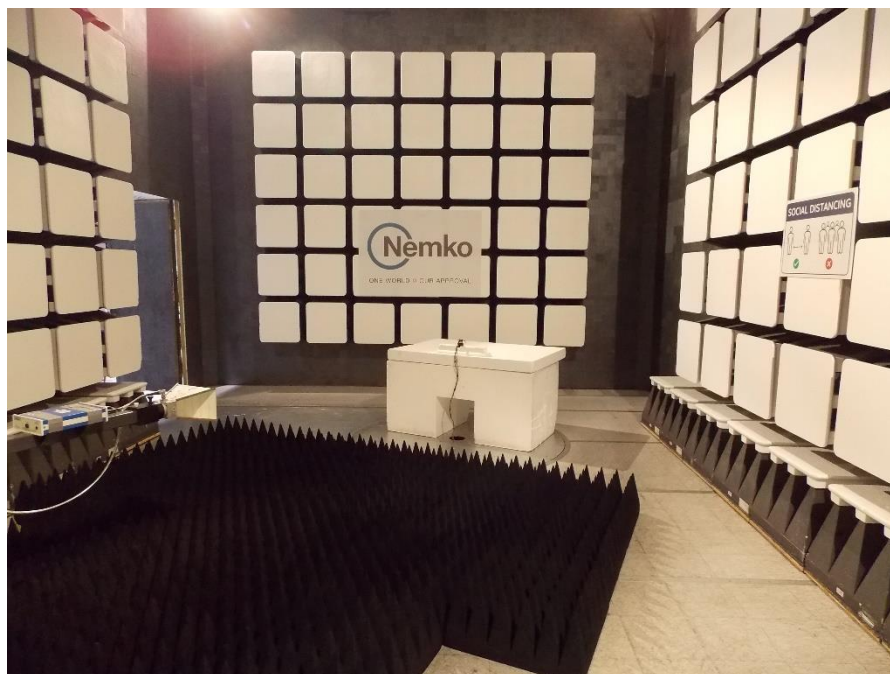
Figure 8.1-8: Radiated emissions setup photo – above 1 GHz
