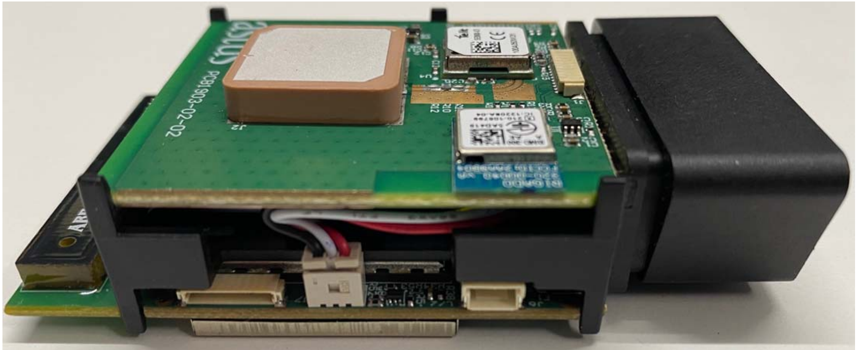
Assembly: Side with the auxiliary connector
