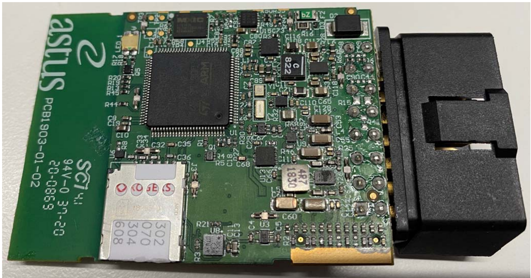
Main board: Bottom (no shield)
