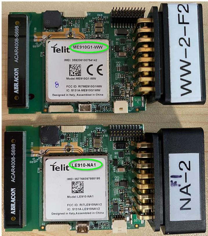
Both radios use the same footprint on the PCB as both have an identical size and pinout.
