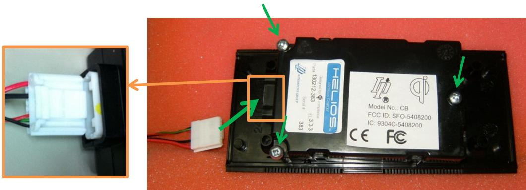
The last step is to attach the connector to the wireless power transmitter, as shown in the picture. Pay particular attention to the orientation of the "clip" on the Helios™ wireless power transmitter and the tab on the mating connector. The picture below shows the whole assembly
