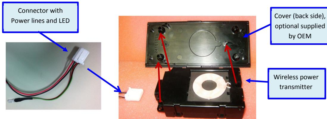
The first step is to attach the wireless power transmitter to the cover by lining them up with the features, as indicated with red arrows in the above picture. Then put screws to the three holes, as shown in picture below, and tight them.
