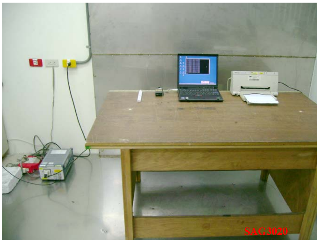
Photo 1: Conducted Emission Test Set-up photo
