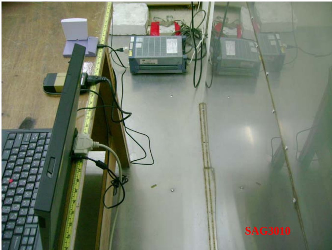
Photo 2: Conducted Emission Test Set-up photo
