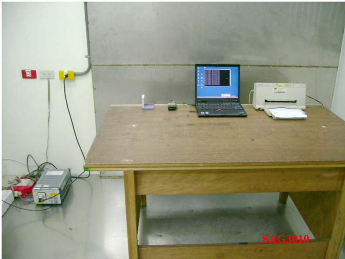
Photo 1: Conducted Emission Test Set-up photo
