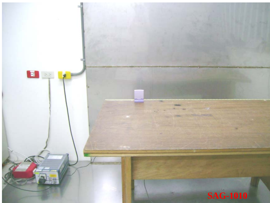
Photo 1: Conducted Emission Test Set-up photo
