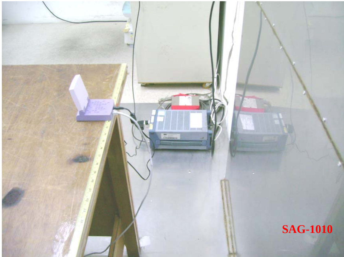
Photo 2: Conducted Emission Test Set-up photo
