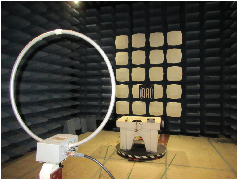
Figure 41: Radiated Measurement Setup, < 30 MHz, Antenna 2
