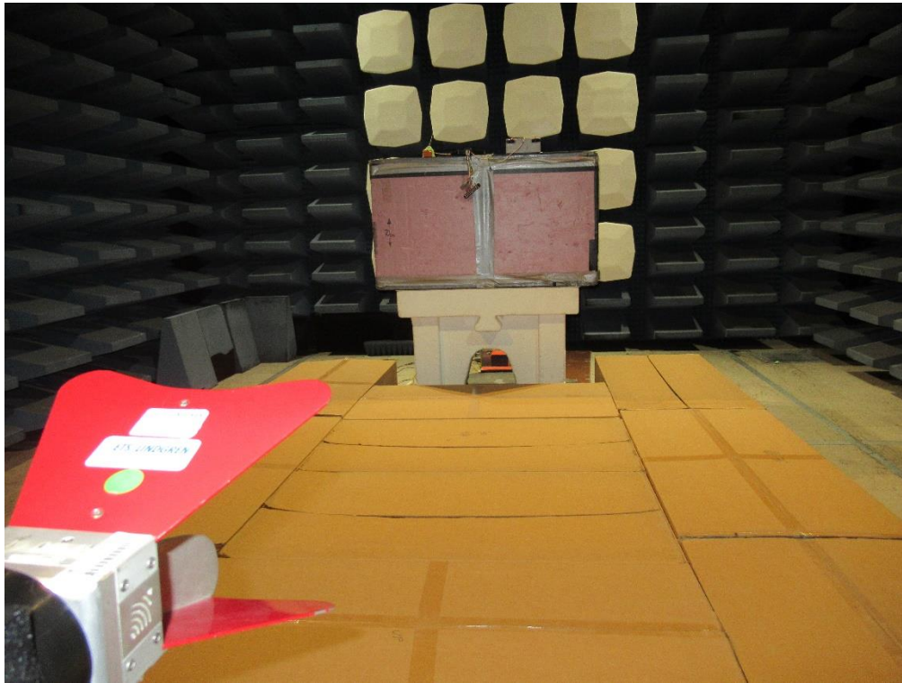
Figure 45: Radiated Measurement Setup, > 1 GHz, Antenna 2
