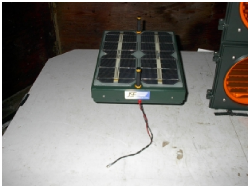
Emission Set up of SZF Module Closeup View Showing Test Cable Bottom & LED
