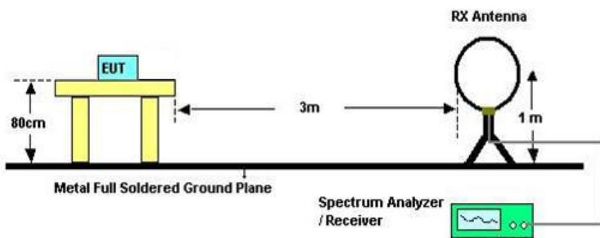
Setup diagram for radiated tests below 1GHz
