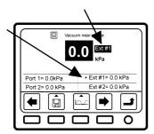
Perform a measurement from the VPR100 unit as described in the Instruction book for VPR100; Chapter Operation. Select external port 1 to use the first registered sensor and extenal port 2 to use the second registered sensor.
