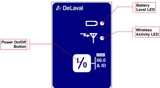
The button is used to turn the sensor on/off and initiate various special functions by holding the button down.
