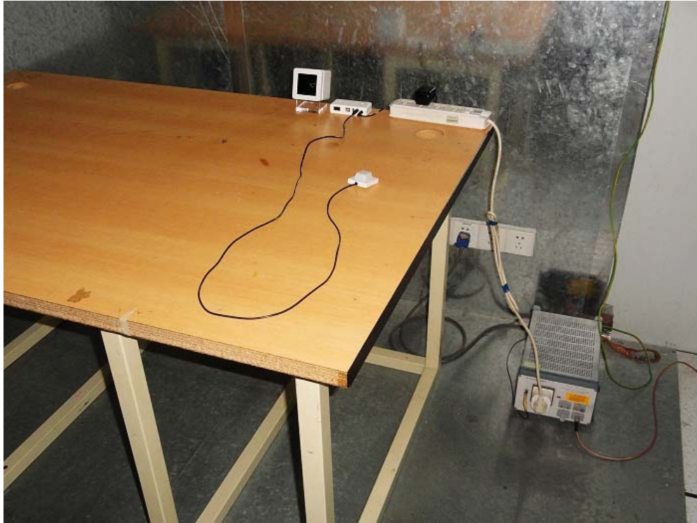
Conducted Emission Test Setup:
