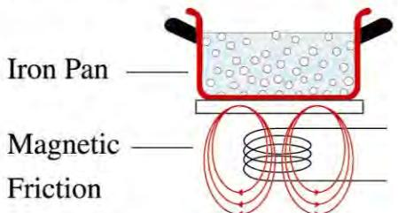
A high frequency (20-35KHz) induction coil underneath the surface ceramic top plate heats the cooking utensil by magnetic friction. The heat is produced directly within the pan. It is controlled by electronic circuit to offer superior performance and functions.
