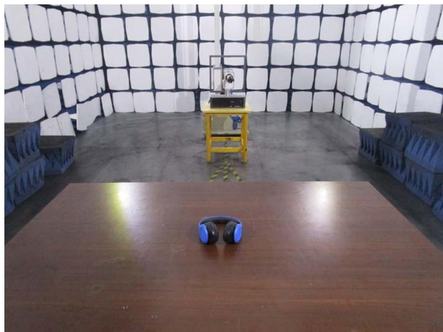
**Radiation Emission Test Setup (30MHz to 1GHz)**
