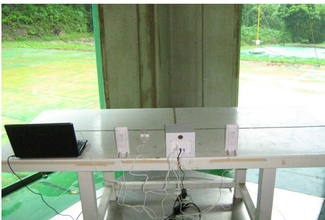
**Above 1GHz Radiated Emission Set up Photos**
