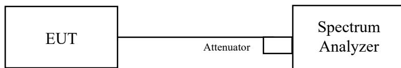
The loss between RF output port of the EUT and the input port of the Spectrum Analyzer has been taken into consideration.
