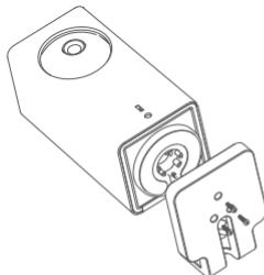
4. Place the bracket onto the two screws previously installed in wall.
