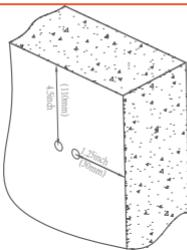
2. For stone, brick and drywall, insert a wall anchor (included) into each hole. Do not use wall anchors if wall is not stone, brick, or drywall. Screw the longer screw into the existing holes or wall anchors. Leave each screw exposed 0.21 inch / 5.0mm out from the wall.
