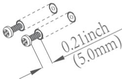
3. Ensure the power cable is plugged in and exits through the base's opening space. Use three short screws to secure the iCamera KEEP to the bracket.
